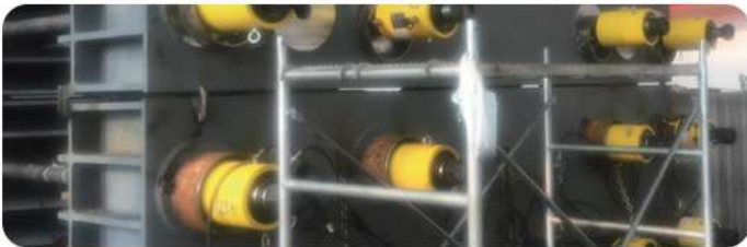
Concrete shield segment loading test
