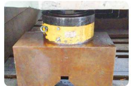
Long term support for large press installation
