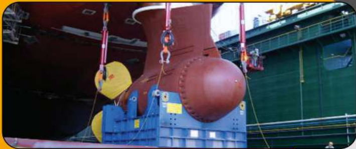
Propeller synchronous lifting installation
