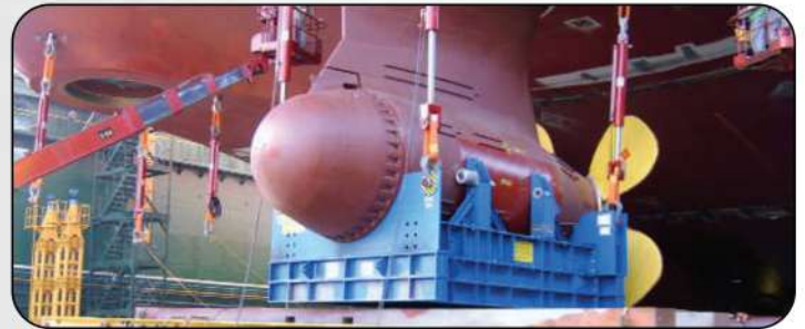
Propeller synchronous lifting installation
