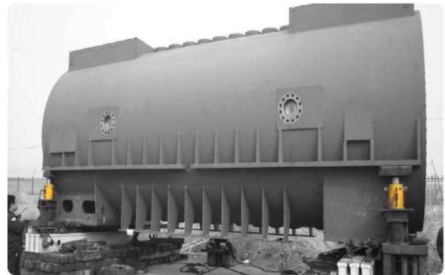
Long-term support for large motor maintenance
