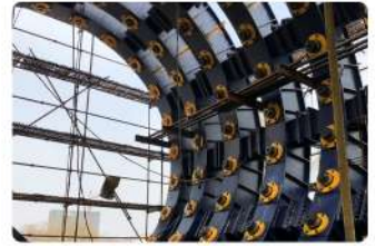
Synchronous loading pressure test of tunnel segment
