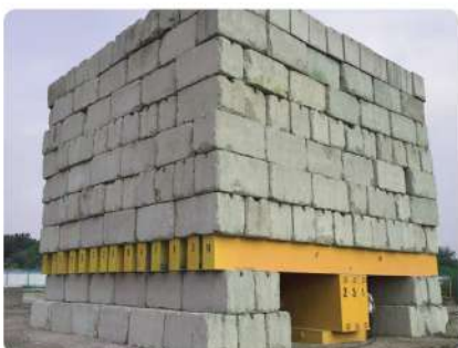
Static load experiment of high-rise building pile foundation
