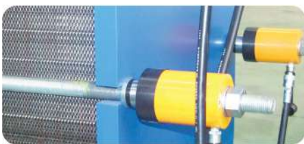
Assembly of large heat exchangers
