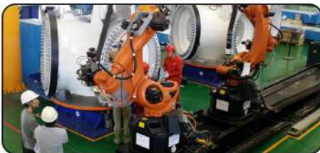
Wind turbine hub assembly
