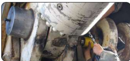
Pusher application for large cylinder disassembly
