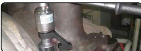
Large pressure vessel bolt pre-tightening
