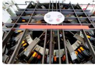
Synchronous loading pressure test of tunnel segment
