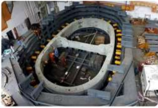
Synchronous loading pressure test of tunnel segment
