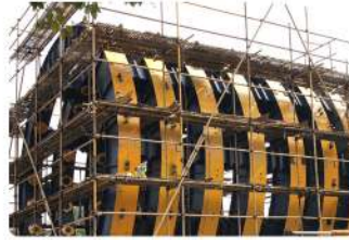
Synchronous loading pressure test of tunnel segment
