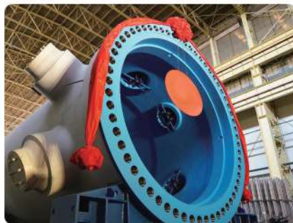
Synchronous lifting and installation of nuclear reactor pressure vessel
