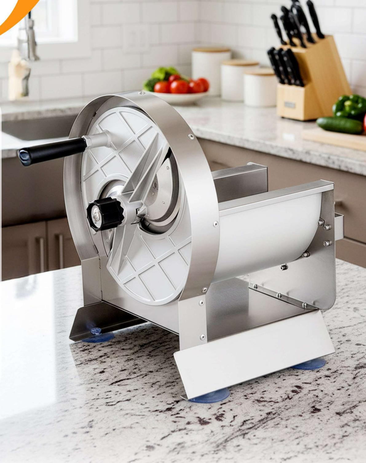
A slicer machine is a cutting machine used to cut ingredients into uniformly sized slices. These machines are often used in the food industry, restaurants, or large kitchens to quickly and consistently cut bread, meat, cheese, vegetables, fruit, and other items.
